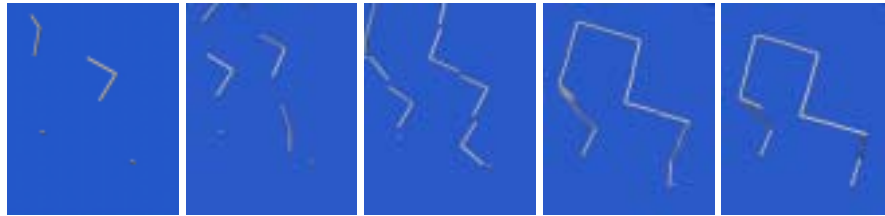
Figure 1: Steps of auto-assembly during optimization for a mechanism with bendy, 90 degree pieces and 2 ground constraints.
