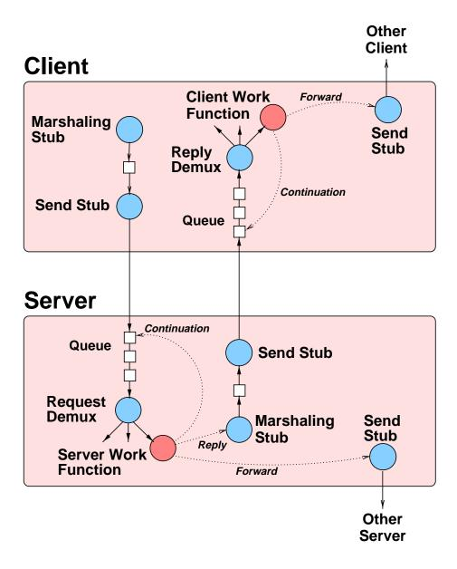
Figure 2: Overview of client/server communication through "decomposed" stubs. Unlike the standard (synchronous RPC) stubs produced by a normal CORBA IDL compiler, Flick's decomposed stubs allow for asynchronous requests and replies, efficient message forwarding, reuse of marshaled messages, and saving intermediate results.
