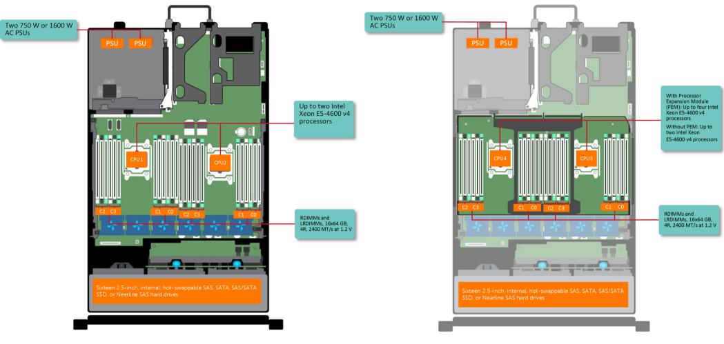
Dell Poweredge R830 System Server with 2 sockets on the main floor and 2 sockets on the expansion
