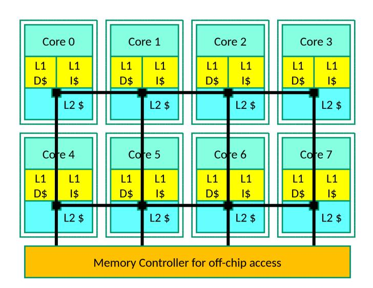
A single tile composed of a core, L1 caches, and a bank (slice) of the shared L2 cache
