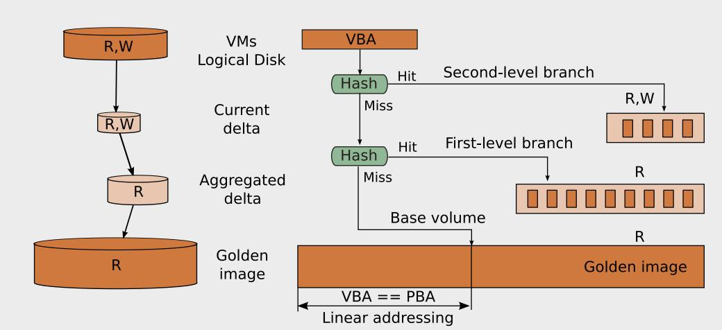
**Translation** of a virtual block address (VBA) to a physical (PBA). Hash table is used for indexing.
