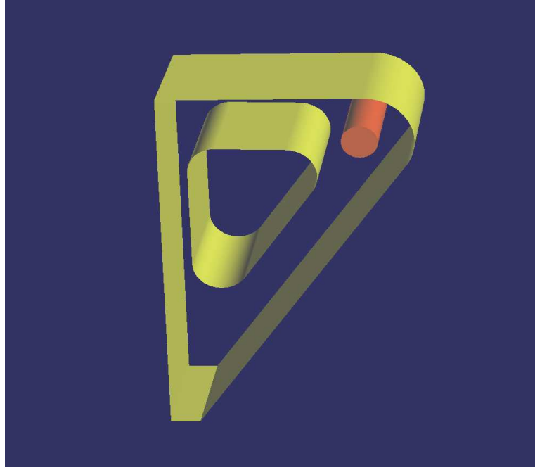
Figure 4.4. Partial model of rocker mount derived from features sketched on the front view of the drawing.
