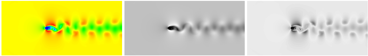
Figure 3. Velocity magnitude. Rainbow (left) and gray scale (middle) color maps were applied to a 2D flow simulation using a spectral element code for solving the incompressible Navier-Stokes Equations. Note how red regions on the rainbow color map are over emphasized while green regions “blur” details that are shown in the gray color map. The image on the right is the decolorized rainbow color map.
