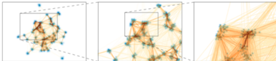
Fig. 1. Application of our visualization technique on a hierarchical data set, zooming from overview (left) to a region of interest (right). The density-based node aggregation field (blue color) guides edge aggregation (orange/red color) to reveal visual patterns at different levels of detail.
