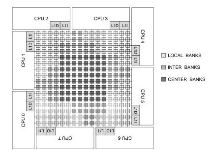
Figure 1. Baseline CMP with 8 cores that share a NUCA L2 cache. The L2 is partitioned into 256 banks and each block is allowed to reside in one of 16 possible banks.
