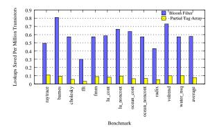
Figure 4. Average messages saved on each L2 access, per million transistors. We compare our filters with an idealized 6-bit partial tag array.
