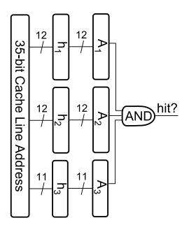
Figure 2. Design of our Bloom filter, showing hash functions  $h_1$  through  $h_3$ , which are used as indexes into bit array slices  $A_1$  through  $A_3$ . A hit is detected when ones are returned from all array slices.
