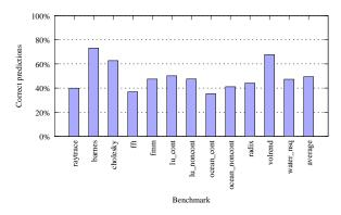
Figure 7. Filter accuracy per L2 access.
