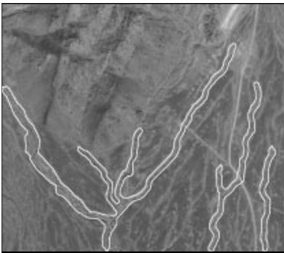
Figure 19: Extracted ravine sides, overlaid onto aerial image.
