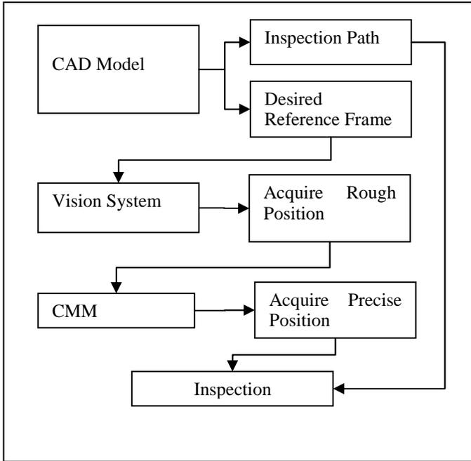
**Figure 3: Integrating the CMM and Vision System**
