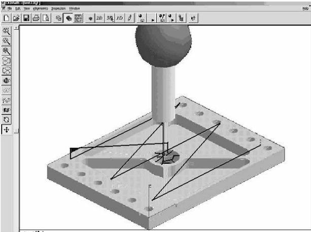
**Figure 5: Inspection Path Planning and Anchor Coordinate System in CadPath**
