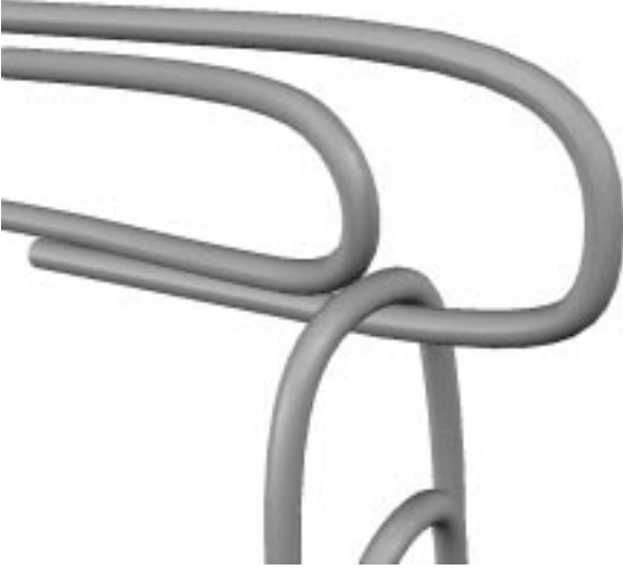
Figure 3: Global considerations are managed through polygonal and numerical tracking methods. Two surface contact constraints are shown in this paperclip example. The global method coordinates with the local, analytic method to add and remove global collision constraints.
