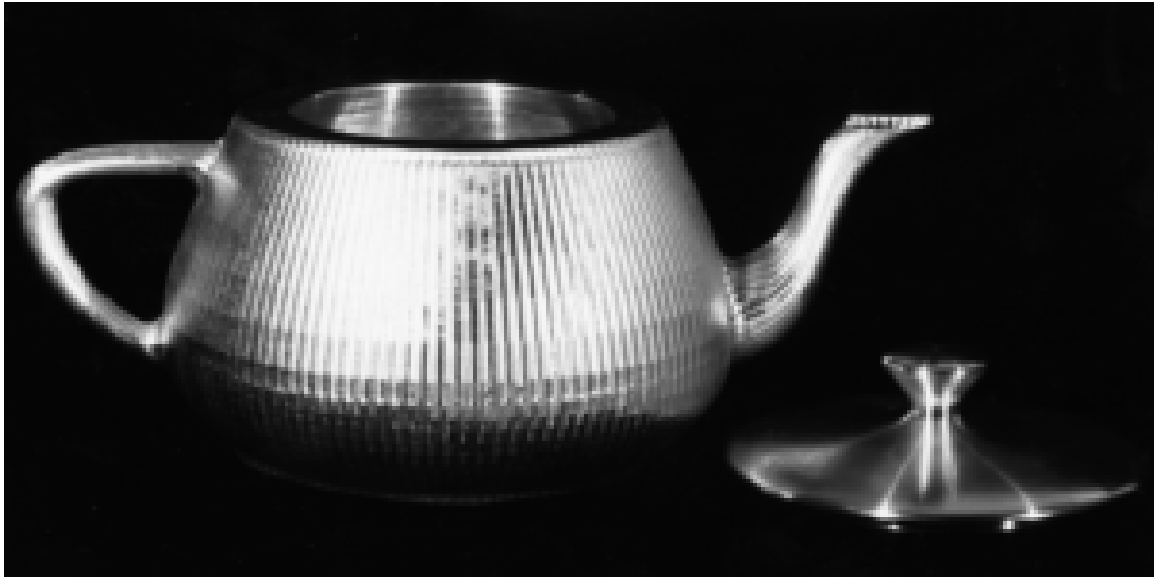
Figure 5: The Utah teapot model, milled using a ball end 3-axis milling.
