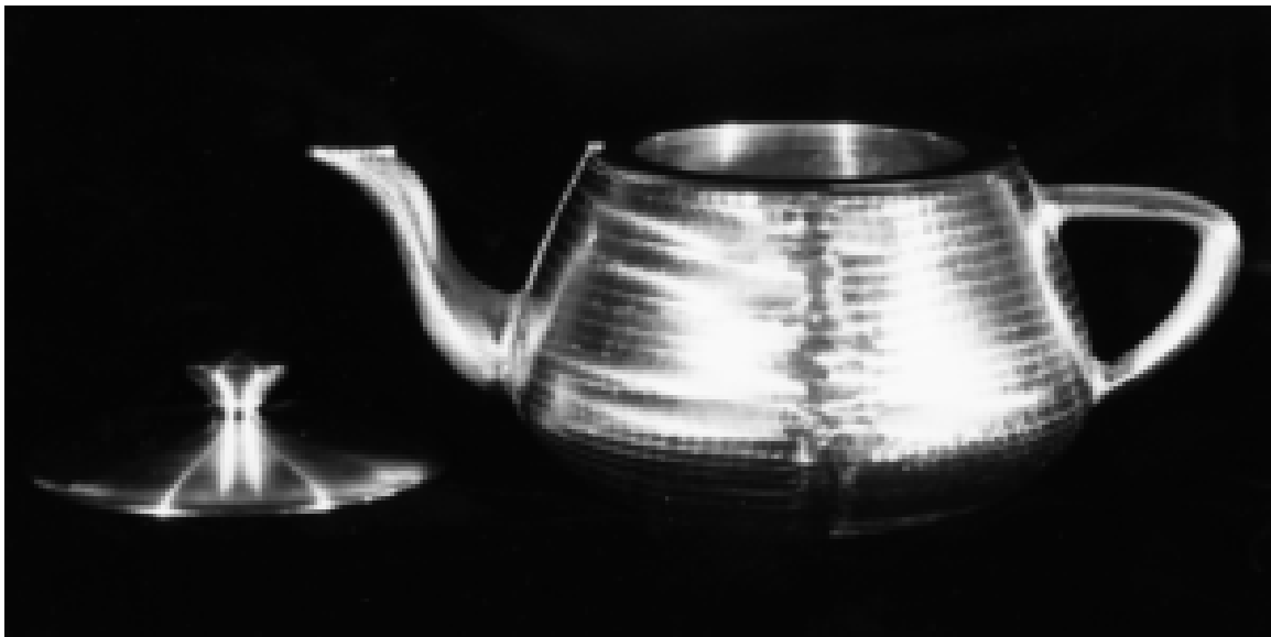
Figure 6: The Utah teapot model, partially milled using a flat end 5-axis milling.
