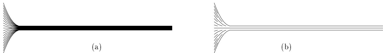
Figure 1: Scan converting complete isocurves can lead to an unbounded amount of redundancy when surfaces are scan converted using isoparametric curves (a). Adaptive extraction of isocurves can introduce much more optimal results (b).
