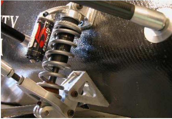
Figure 4. A rocker mount and its associated assembly.
